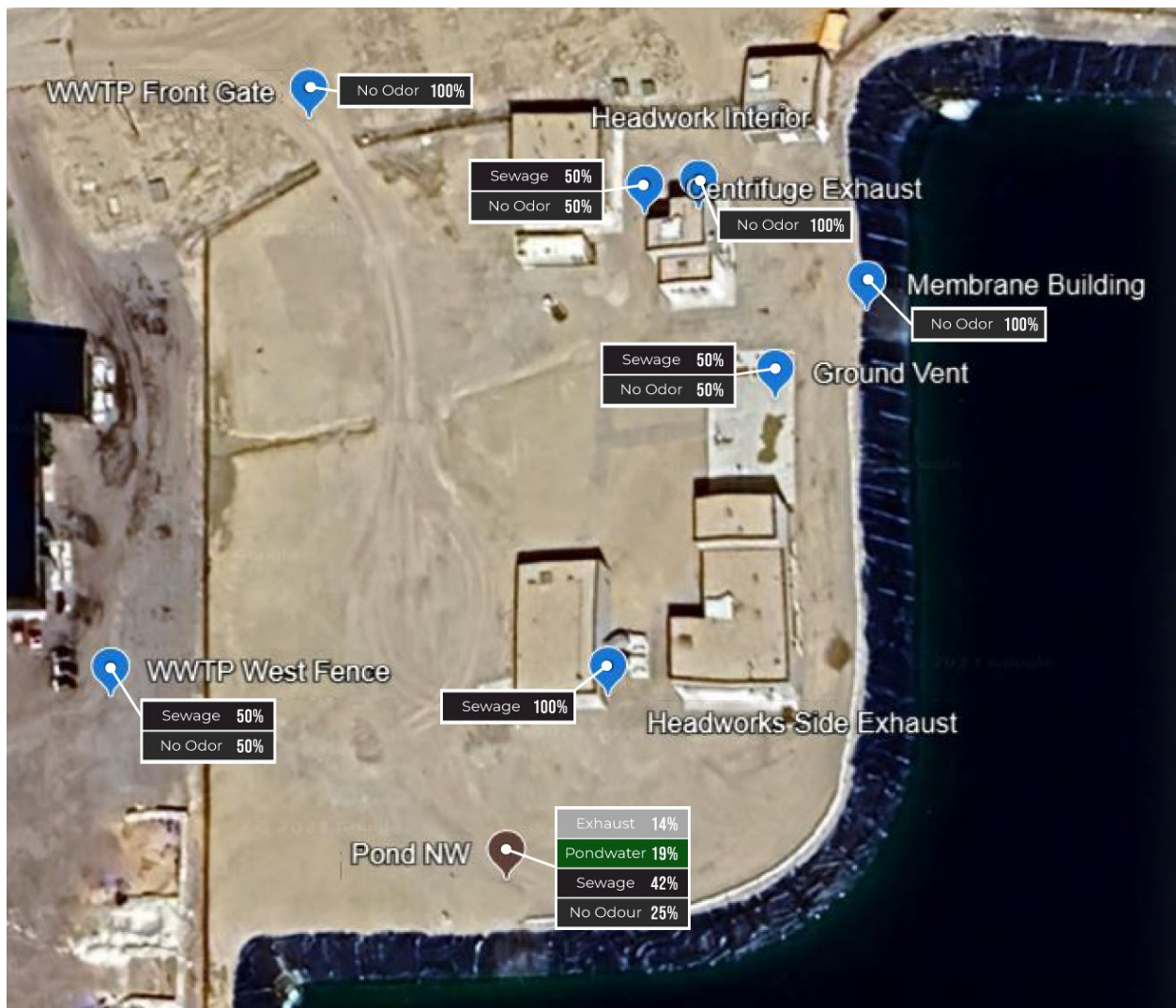
Figure 8: Percentage of Encountered Odours at Each Sampling Point within the WWTP
